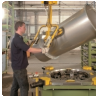
Strong in series: Quality flanging for XL pipes up to DN 800 mm.
