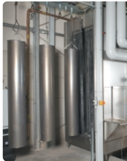
Quality control - High-quality powder-coated pipes leave the spray cabin.
